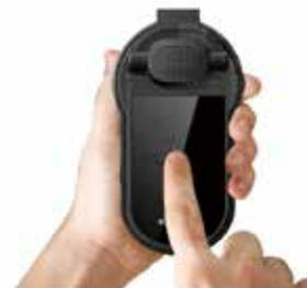
The DSJ-U1 is integrated with a shortcut button and touchscreen which make it more user-friendly. Shortcut buttons, including "PTT", "Power On/Off", "Video Recording", "Audio Recording", "Snapshot", "Event Tag", "Volume Up/Down", can be used for all kinds of rapid operations. (Some of the buttons are reserved for more extensive applications). All of its settings and operational capabilities can be accessed visually through its 2.2-inch touchscreen.
