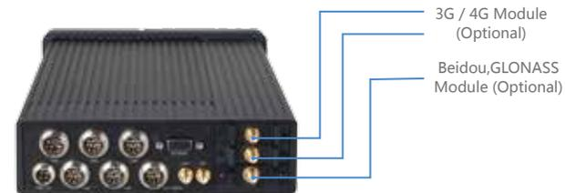
The embedded GPS, WiFi module and optional global position module such as Beidou, GLONASS in the KDM2410M-V21 can upload the vehicle's accurate location to command center. Optional 3G/4G module makes it possible to support almost all kinds of network protocols, including FDD-LTE, TDD-LTE, HSPA/UMTS, GSM/GPRS/EDGE, TD-SCDMA, EVDO/CDMA and so on. Video stream can be transmitted to command center instantly with such diversified network adaptability.
