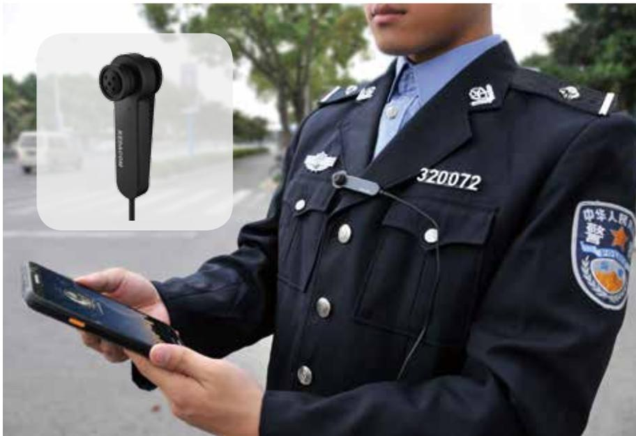
USBCAM-100 is an external USB camera which can be used together with IPW200 and DSJ-U1. It can be disguised as a button and used for covert surveillance. It weighs just 30 grams which is conveniently worn with service uniforms.
